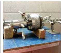
Fugitive Emission Gas testing
