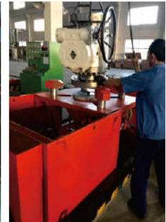
Hydrostatic Testing Picture
